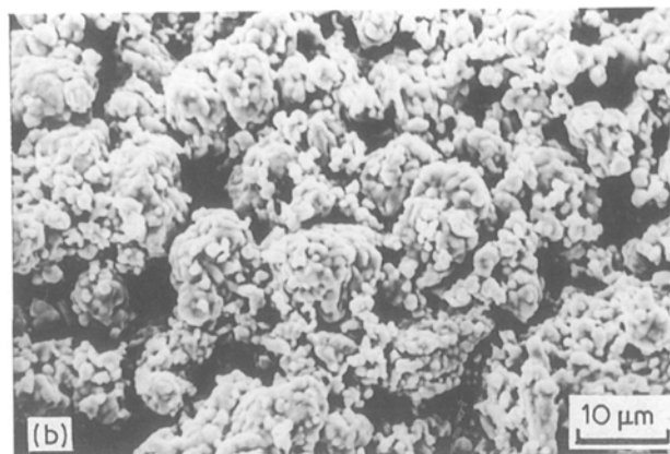
Figure 8 Scanning electron micrographs of \text{Cd}_{1.9}\text{Pb}_{0.1}\text{SnO}_4 fired thick films. (a) 500°C, (b) 700°C and (c) 900°C.
